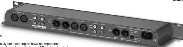
The four XLR-3 electronically balanced inputs have an impedance of  $20k\Omega$  bridging and are routed to four unbalanced RCA (phono) outputs with an output impedance of  $<50\Omega$ .
