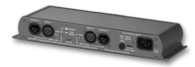
The rear panel mode switch changes the unit from dual mono to stereo, when only the pre-sets for channel 1 (left) are active and apply to both channels. Stereo limiting operates by limiting both left and right outputs if either left or right input needs to be limited. Dual mono limiting operates by limiting left and right signals individually, so you can use the RB-SL2 as two separate mono limiters.
