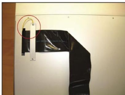
Fig 2-14 : Mixer Bus Cable Screen Connection.
